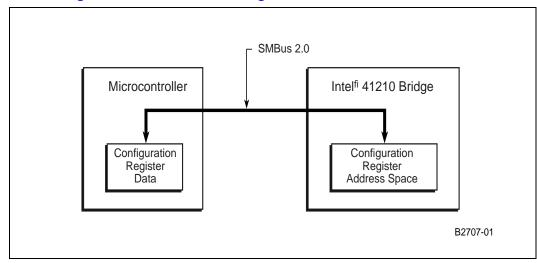
Figure 1. 41210 Bridge Microcontroller Block Diagram
